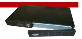
As long as utility power is present, the batteries can be hot swapped without interrupting power to connected equipment. The process of swapping out the batteries does not require special equipment. Simply pull the front cover off and remove the internal battery pack holder with a Phillips screwdriver. Slide the front-load battery packs out of the UPS and then slide the new battery pack into the UPS unit and secure.
